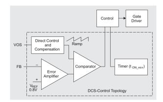
Figure 1. Block diagram of the DCS-Control topology.
