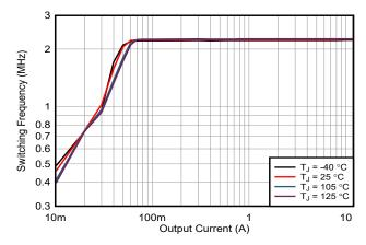
*Figure 5.* Switching frequency variation of the TPSM8287A12 power module with fixed-frequency DCS-Control.
