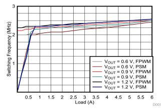
*Figure 4.* Switching frequency variation of the TPS62869 with DCS-Control.
