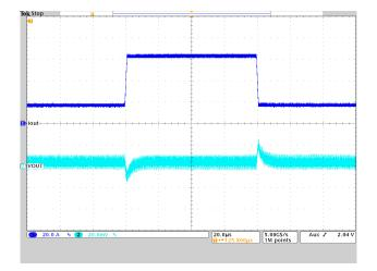
**Figure 3.** The transient response of fixed-frequency DCS-Control is tunable to the most severe load transients, where it provides excellent regulation.
