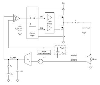
*Figure 2.* Block diagram of the TPS62873's fixed-frequency DCS-Control topology with the oscillator, differential remote sensing, transconductance amplifier and hysteretic comparator.
